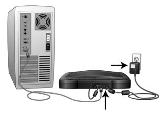
**Note**: Your scanner does not have a power switch. Plugging it in turns on the power.
